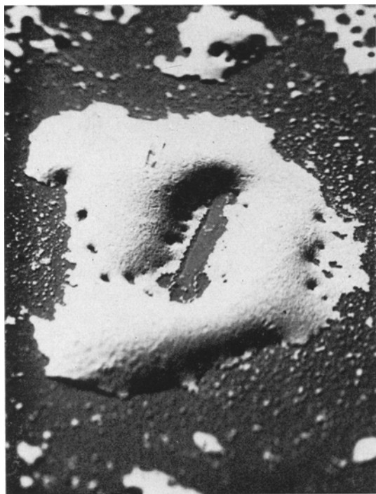
Figure 3 Drops of evaporated lead not completely wetting the aluminium surface ( \times 200 ).
